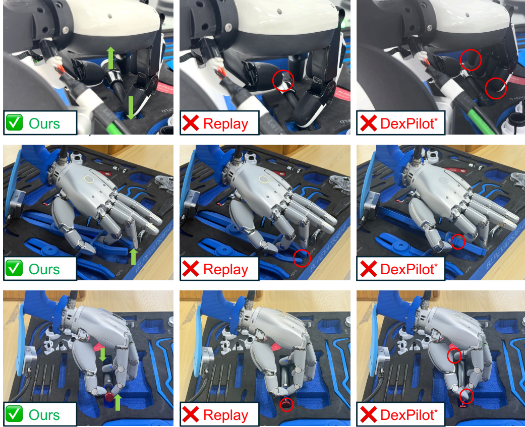
Figure 5: Failure analysis for hand motion control. Representative hand-control outcomes compare the residual hand skill, kinesthetic replay, and DexPilot* across contact-rich manipulation cases.
