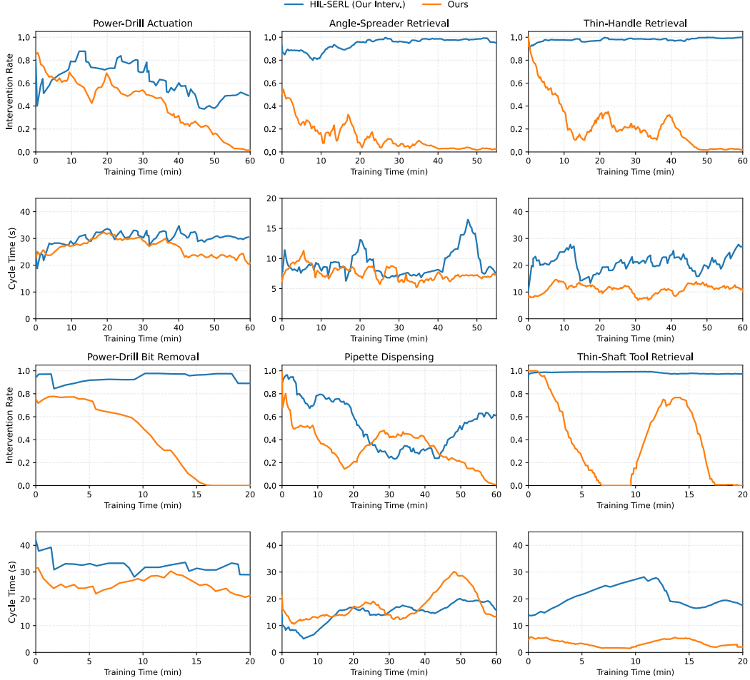
Figure 3: Online training curves across six tasks. For each task, intervention rate (upper) and cycle time (lower) are shown as running averages over 20 episodes, comparing our method (Ours) against the HIL-SERL (Ours Interv.) baseline. Lower intervention rate indicates more autonomous execution, while lower cycle time indicates more efficient completion.
